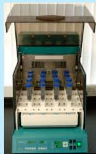
CTRL-16 brushing simulator consisting of a specimen bath and brushing rig assembled inside a Jeiotech SI300R incubator shaker unit.
